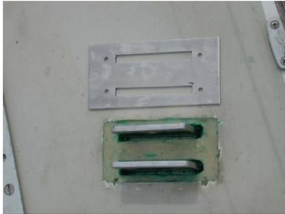
Have a new chain plate cover made that is about 4" X 8" and 1/8" thick. Make two plywood templates with the slots 3/32" to 1/8" clear around the chainplates. Note that I found that the chainplates are NOT exactly parallel nor the same distance apart. Be sure to mark the top side of each template. The holes should be 1/2 the distance from the chainplate to the edge of the new cover.
