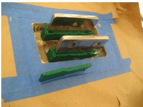
Buy a block of kid's modeling clay. Cut strips that are 1" high and 1/4" to 5/8" thick and carefully press them against the chain plates being careful that they go all the way to the lower surface and are at least as high as the top deck surface.
