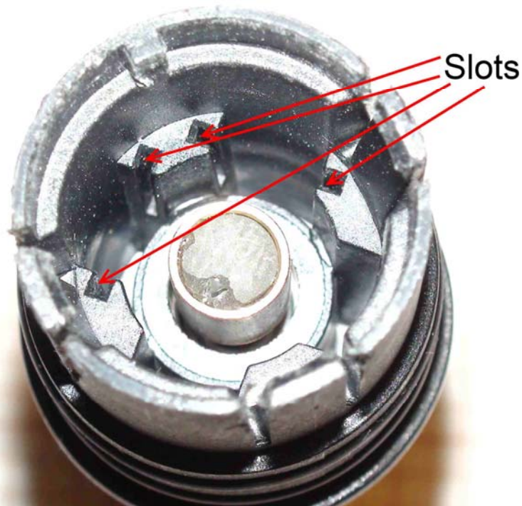
Module Housing showing the slots for the magnetic pickups.
