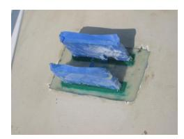
Before you remove the craft paper, do a rough grind of the surface of the epoxy be be sure there are no really low spots.
