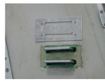
Have a new chain plate cover made that is about 4" X 8" and 1/8" thick. Make two plywood templates with the slots 3/32" to 1/8" clear around the chainplates. Note that I found that the chainplates are NOT exactly parallel nor the same distance apart. Be sure to mark the top side of each template. The holes should be  $\frac{1}{2}$  the distance from the chainplate to the edge of the new cover.
