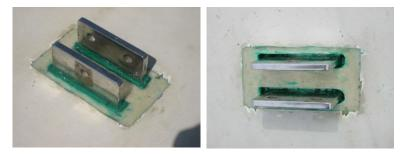
Put the new covers in place and tape the deck up to the edges. Then remove the cover and inject the caulking (Sikaflex or 3M 4200) into the spaces by the chainplates being as careful as possible to totally fill the spaces all the way down. Then cover most of the surface of the epoxy with a thin coat of the same caulking. Put the cover on and screw it down.
